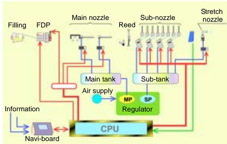
**Figure 1:** Filling feeding system
