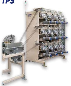
Optional off-machine winder for TPS prepreg slitter to rewind narrow slit tapes with widths such as 1/8", 1/4", 1/2", 1". Bobbin traverse system is adopted. Each tape tension is controlled individually by TSUDAKOMA's original tension control technology. Liner film unwinder is employed to rewind thermoset prepreg tape, used on the Automated Fiber Placement (AFP).
