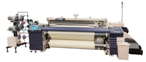
The ZAX9200*i* realizes highspeed stability in weaving and reduces air consumption by 10% with its clear shedding due to the new shortened beating stroke, the *i*-Weave, and the DSS-II Direct Subnozzle System.
