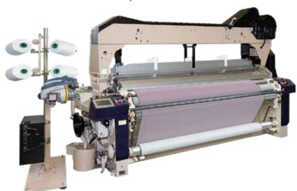
High-speed and stable operation of the ZW508 will be demonstrated with a reed space of 230 cm increasingly demanded. It weaves a wide range of fabrics from general apparel fabrics to middle-thick value-added fabrics with the lowest running costs.
