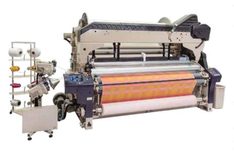
TSUDAKOMA has addressed environmental issues for many years. The ZW8100 increases its speed by 10 % while reducing electric power consumption by 5 % and on-loom vibration by half compared with conventional models. Furthermore, high valueadded fabric weaving is possible. Our water jet loom weaves high value-added fabric with multicolor and top & bottom double beams at high speeds. The new nozzle achieves stable 4-color weft insertion and reduces water consumption by 10 %.
