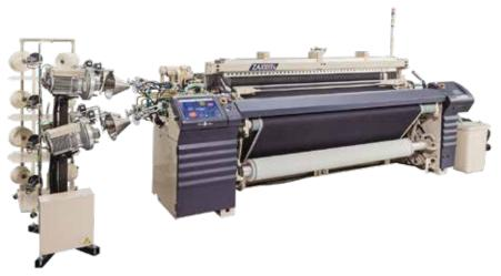
In the Chinese market, TSUDAKOMA will focus on highlighting air jet looms capable of weaving denim. Air jet looms are presently the mainstream of denim weave worldwide. The ZAX9200*i* enhances productivity and weaves high-quality denim even at high speeds. The adjustable guide bar greatly reduces the time it takes for style change. It is no longer necessary to cut the guide bar to match the reeding width.
