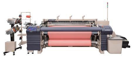
The ZAX9200*i* MASTER shows its full abilities of high-speed, air-saving, and stable performance. It supports design-rich high quality fabric which satisfies diversified life styles and the fashion-conscious. The ZAX9200*i* MASTER weaves a fabric with extensive range of kinds and thicknesses using positive electronic dobby.
